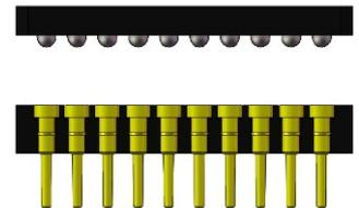
Standard SMT pin, raised SMT pin and SMT solderballs are available in both functions.
