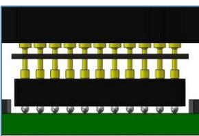
Most of the E-tec Interconnect Test Sockets can be transposed on a SMT adapter, with excellent efficiency and reliability.
