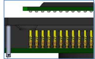
The solderless socket is easily mounted to the PCB with 2, 4 or 8 through hole mounting pegs. The assembly board ensures perfect coplanarity of the socket. Contact reliability is guaranteed with spring loaded gold plated contacts, which are pressed onto gold plated PCB pads. Solderless compression type sockets are available with all retention systems. Our goal is to solve your requirements - many different terminals and configurations are available.
